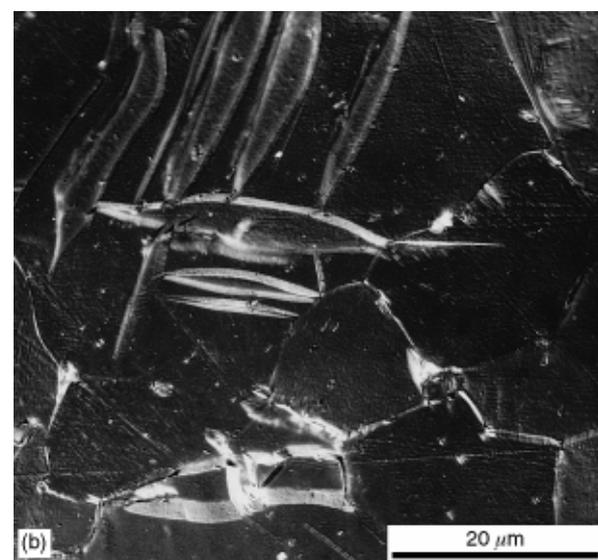
Figure 4 Fatigue microcracks near twins, (a) fatigue crack along twin boundary, (b) fatigue crack by interaction of twins.
