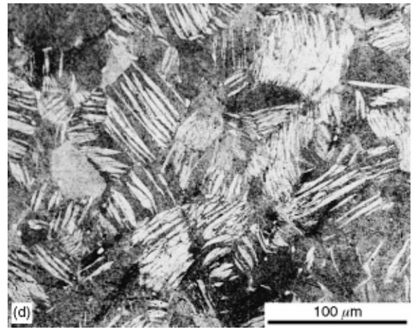
Figure 2 Deformation twins at  $\epsilon_a = 2.4\%$ , (a)  $N = 3$  cycles, (b)  $N = 10$  cycles, (c)  $N = 50$  cycles, (d)  $N = 100$  cycles.
