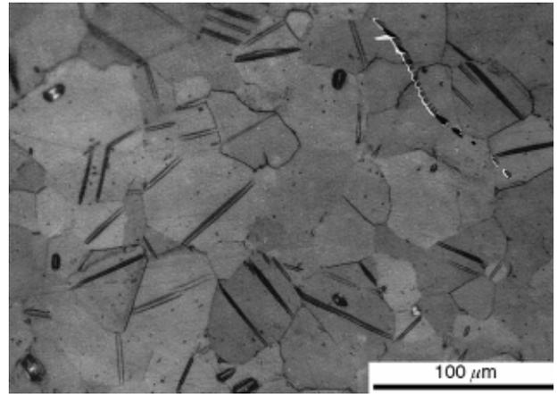
Figure 3 Deformation twins at  $\epsilon_a = 1.5\%$ .
