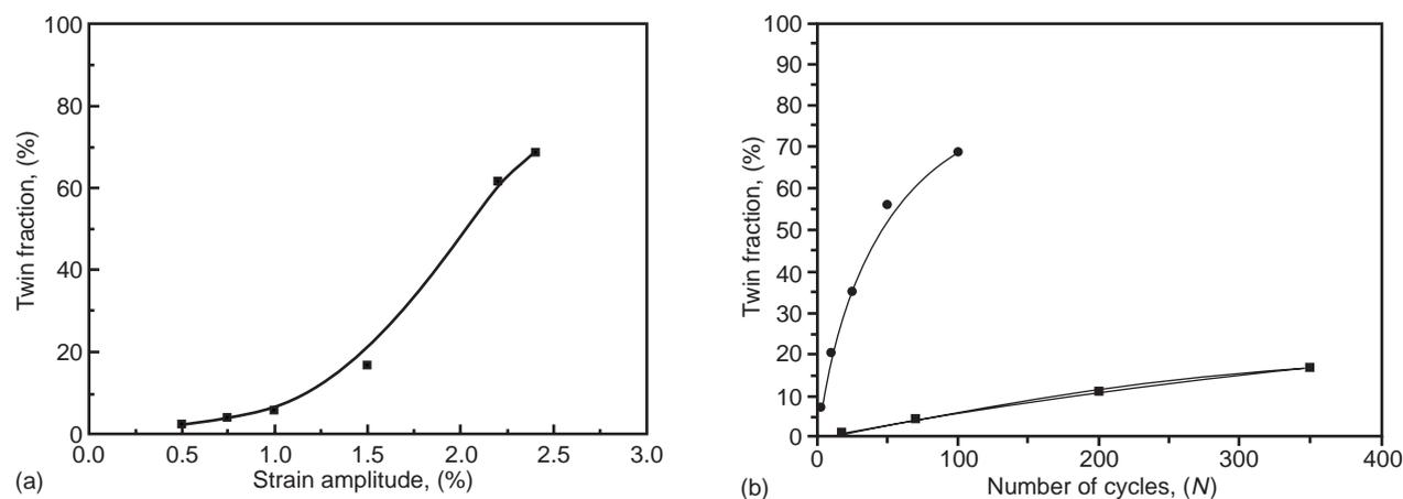
Figure 1 The influence of strain amplitude and number of cycles on deformation twinning in commercial purity titanium, (a) relation of twin fraction to cyclic strain amplitude, (b) relation of twin fraction to number of cycles, (●) 2.4%, (■) 1.5% strain.
