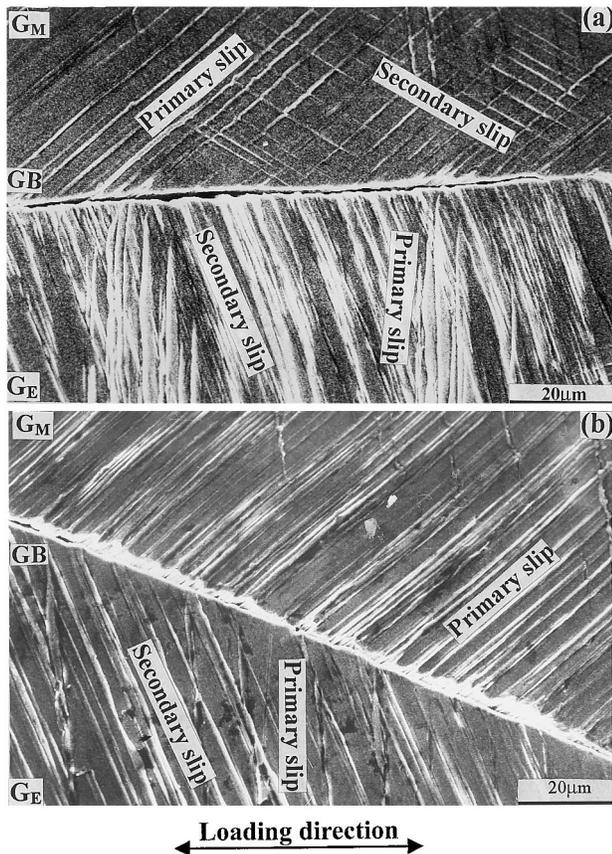
Fig. 4. Fatigue cracking along the GB segment from A, B, C, to D. (a) Fatigue cracking at the site B; (b) fatigue cracking at the site C.
