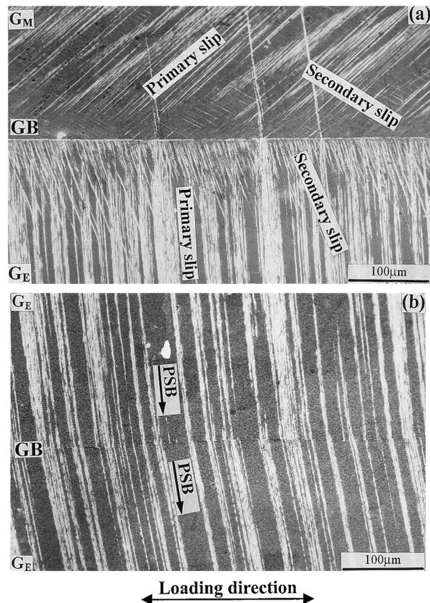
Fig. 3. Surface slip morphology near the GBs in the bicrystal. (a) At the site B of the GB segment; (b) at the site F of the GB segment.
