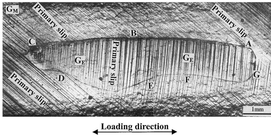
Fig. 2. Surface slip morphology of the bicrystal cycled at the axial plastic strain amplitudes of  $2.2 \times 10^{-4}$  for  $2 \times 10^4$  cycles,  $5.4 \times 10^{-4}$  for  $5 \times 10^3$  cycles,  $1.0 \times 10^{-3}$  for  $3 \times 10^3$  cycles and  $1.5 \times 10^{-3}$  for  $2 \times 10^3$  cycles, respectively.
