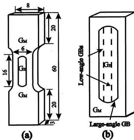
Fig. 1. Fatigue specimen of the bicrystal. (a) Geometrical dimension of the bicrystal; (b) constitution of the component crystals in the gauge part of the bicrystal.
