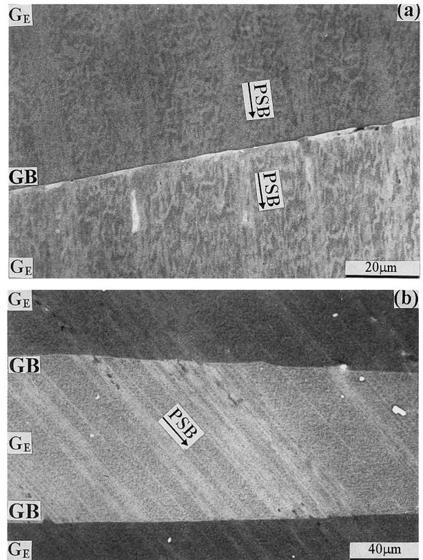
Fig. 7. Dislocation patterns near GB segment from D, E, F, to G observed by the SEM-ECC technique. Micrographs (a) and (b) PSBs transferring through the GB continuously.
