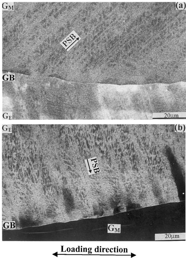
Fig. 6. Dislocation patterns near the GB segment from A, B, C, to D observed by the SEM-ECC technique. Micrographs (a) and (b) showing discontinuous distribution of dislocations beside the GB.
