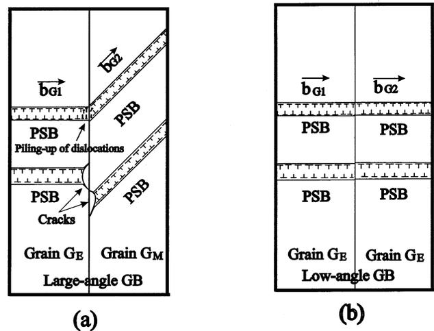
Fig. 8. Interaction modes of PSBs with large- and low-angle GBs. (a) Interaction of PSBs with a large-angle GB, showing the intergranular cracking by piling-up of defects; (b) interaction of PSBs with a low-angle GB, showing the passing-through of defects.
