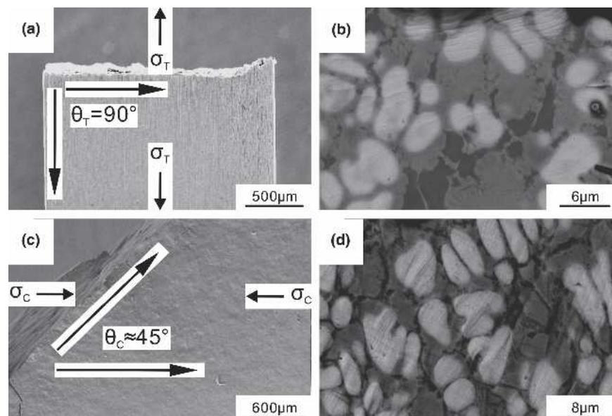
FIG. 3. SEM micrographs revealing deformation and fracture features of Ti-based composite under (a) and (b) tensile loading; (c) and (d) compression loading.
