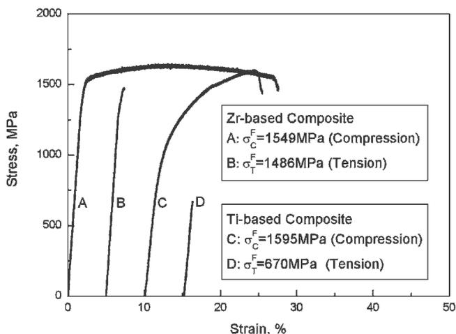
FIG. 1. Tensile and compressive true stress-strain curves of Zr- and Ti- based composites at a strain rate of  $10^{-4} \text{ s}^{-1}$ .
