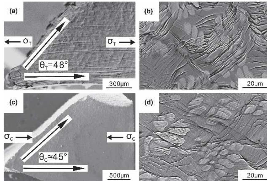
FIG. 2. SEM micrographs revealing deformation and fracture features of Zr-based composite under (a) and (b) tensile loading; (c) and (d) compression loading.
