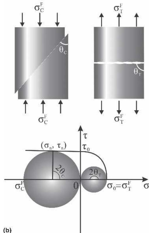
FIG. 4. Illustration of critical tensile and compressive failure conditions at (a)  $0 < \alpha = \tau_0/\sigma_0 < \sqrt{2}/2$  for Zr-based composite and (b)  $\alpha = \tau_0/\sigma_0 \geq \sqrt{2}/2$  for Ti-based composite.
