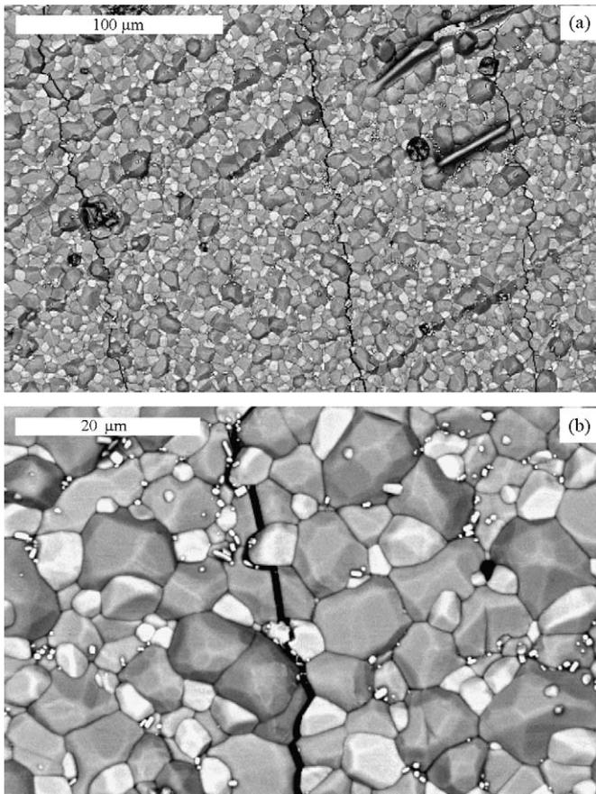
Fig. 6. SEM-second electron micrographs of the crack propagation within the  $\text{Cu}_6\text{Sn}_5$  IMC layer: (a) straight propagation path and (b) intergranular and transgranular manners.
