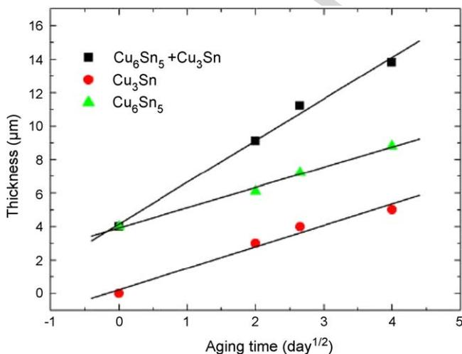
Fig. 3. Dependence of the thicknesses for the IMC layers at the SnAgCu/copper single crystal joint on the aging time at 170 °C.
