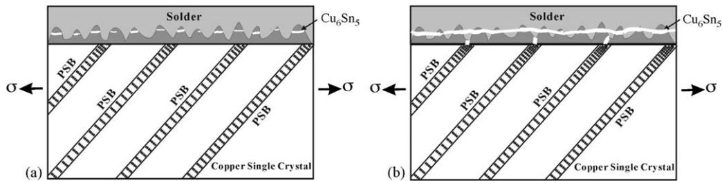
Fig. 7. Illustration of the damage process at the as-reflowed interface under the interaction of PSBs with the interface: (a) fracture of the protrudes of IMC and (b) cracking at the intersection site of PSBs with the interface and failure along the interface of solder/IMC layer.
