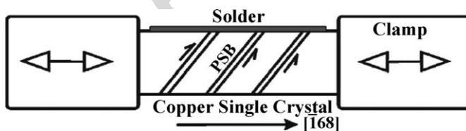
Fig. 1. Illustration of the fatigue specimen with an IMC interface between the solder and copper single crystal.
