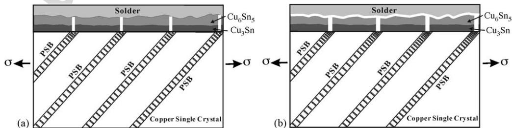
Fig. 8. Illustration of the damage process at the aged interface under the interaction of PSBs with the interface: (a) cracking at the intersection site of PSBs with the interface and (b) failure along the interface of solder/IMC layer.
