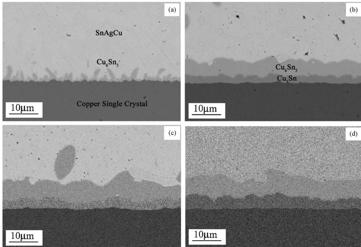
Fig. 2. SEM-backscattered electron micrographs of the morphology of IMCs at the SnAgCu/copper single crystal interface: (a) as-reflowed, (b) aged at 170 °C for 4 days, (c) 7 days, and (d) 16 days.
