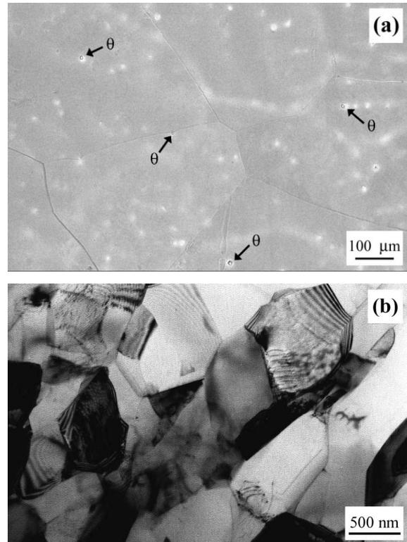
Fig. 2. Microstructure of cast alloy Al-0.63%Cu, (a) and TEM images showing the microstructure of Al-0.63%Cu alloy ECAPed for four passes (XZ-plane), (b).
