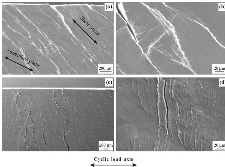
Fig. 9. Shear bands on the surface of the specimen ECAPed for four passes and fatigued to failure under plastic strain amplitude of  $10^{-3}$ . (a) and (b) observed on XZ-plane, (c) and (d) observed on XY-plane.
