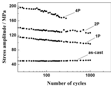
Fig. 3. Cyclic stress response of Al-0.63%Cu alloy subjected to different numbers of ECAP passes indicated as "1P, 2P, 4P", fatigued under a constant plastic strain amplitude of  $10^{-3}$ .
