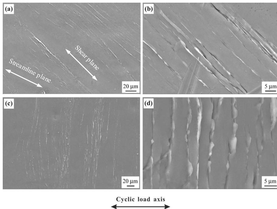
Fig. 7. Shear bands on the surface of the specimen ECAPed for one pass and fatigued for 1000 cycles under plastic strain amplitude of  $10^{-3}$ . (a) and (b) observed on XZ-plane, (c) and (d) observed on XY-plane.
