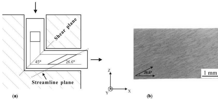
Fig. 10. Illustration of streamline structure forming, (a) illustration of the ECAP process, (b) SEM micrograph of the Al-0.63 %Cu alloy ECAPed for one pass (XZ-plane).
