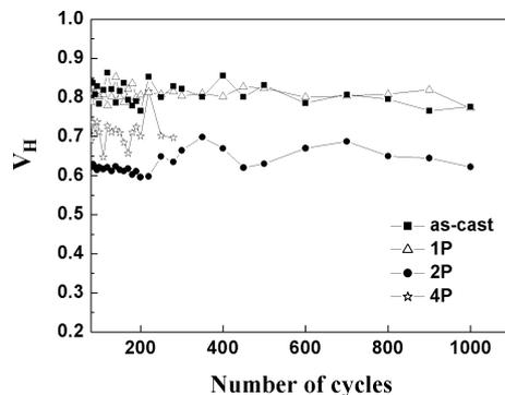
Fig. 5. Variation of shape parameter of the specimens subjected to different numbers of ECAP passes, fatigued under a plastic strain amplitude of  $10^{-3}$ .
