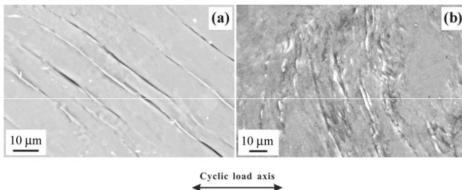
Fig. 11. Shear bands on the surface of the rolled pure Al specimen fatigued for 5000 cycles under plastic strain amplitude of  $10^{-3}$ , observed on (a) XZ-plane and (b) XY-plane.
