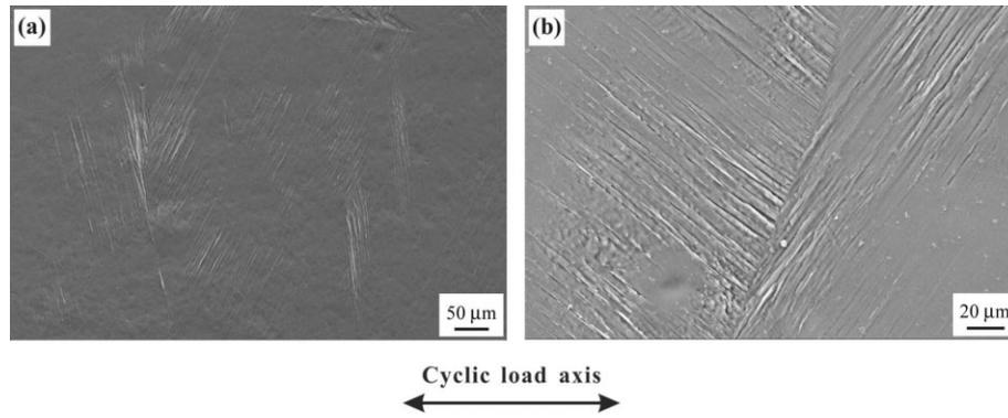
Fig. 6. Surface morphology of the as-cast Al-0.63%Cu alloy fatigued for 1000 cycles under plastic strain amplitude of  $10^{-3}$ .
