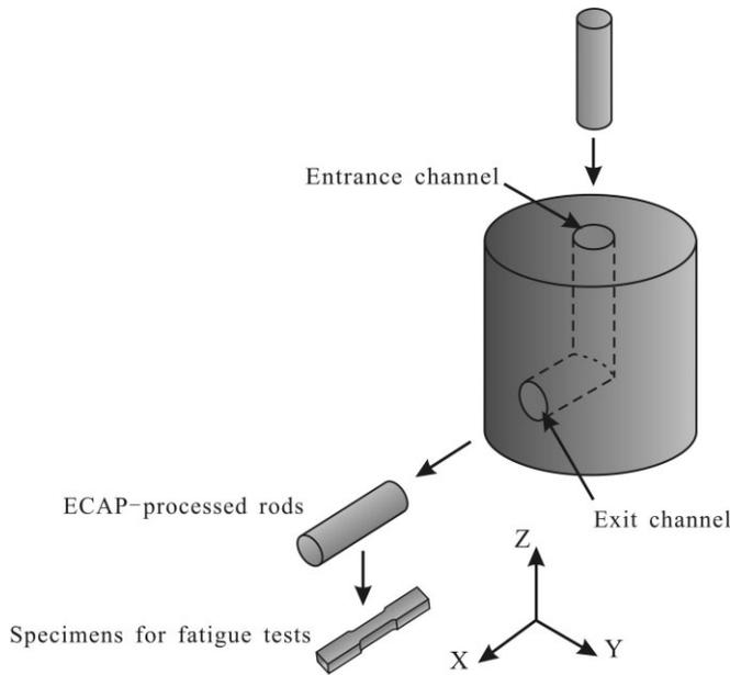
Fig. 1. Illustration of ECAP die and orientation of fatigue specimens relative of the pressing direction.
