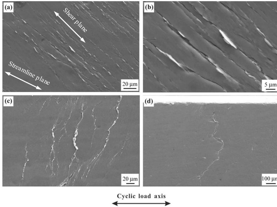
Fig. 8. Shear bands on the surface of the specimen ECAPed for two passes and fatigued for 1000 cycles under plastic strain amplitude of  $10^{-3}$ . (a) and (b) observed on XZ-plane, (c) and (d) observed on XY-plane.
