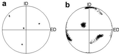
**Figure 1.** Pole figures for crystal II: (a) initial orientation; (b) after one-pass ECAP (ID, insertion direction; ED, extrusion direction).
