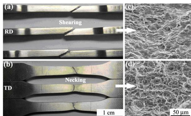
**Figure 4.** Macroscopic and microscopic tensile fracture features of the RD and TD samples.
