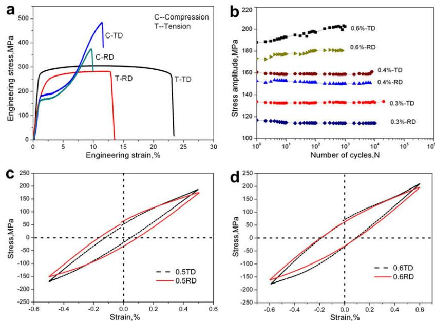
Figure 2. (a) The tensile and compressive stress–strain curves of the samples in the TD and RD at a strain rate of  $5 \times 10^{-3} \text{ s}^{-1}$ ; (b) cyclic stress responses of the TD and RD samples at total strain amplitudes of 0.3, 0.4 and 0.6%; (c and d) hysteresis loops of the RD and TD samples at total strain amplitudes of 0.5% and 0.6%, respectively, at the first and after several circles.
