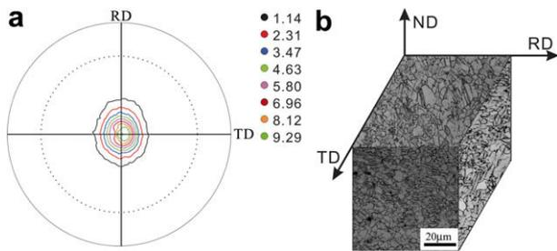
Figure 1. (a)  $\{0002\}$  pole figure for rolled AZ31 alloy; (b) optical images of the microstructures observed in three planes.
