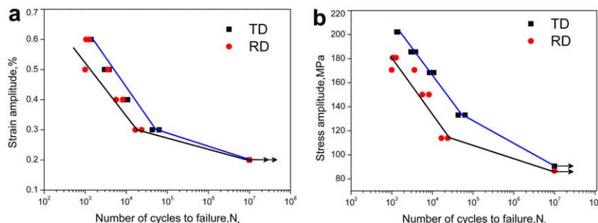
**Figure 3.** (a) Total strain amplitude as a function of the number of cycles to failure for the RD and TD samples; (b) stress amplitude vs. number of cycles to failure curves for the RD and TD samples.
