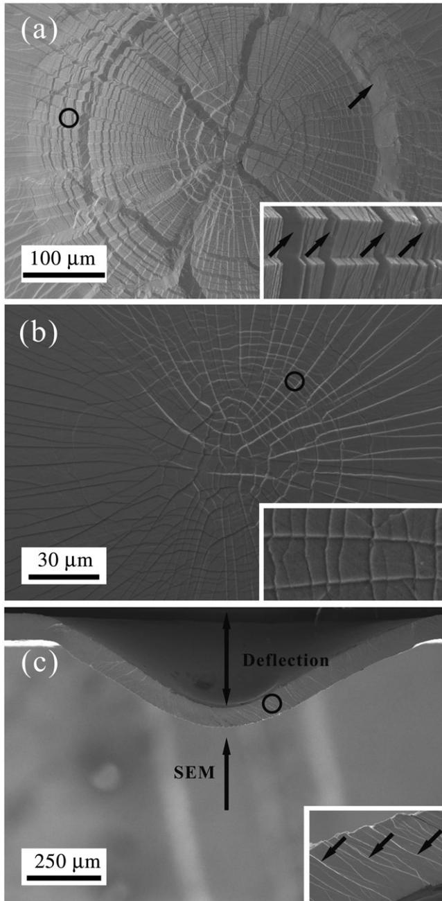
Figure 1. (a) Morphology of the shear band pattern on the lower surface of Pd-based metallic glass punched at a deflection of 0.45 mm as a typical example for ductile MMG (a); (b) for macroscopically brittle Fe-based metallic glass punched at a deflection of 0.15 mm; and (c) morphology of the cross-sectional plane of Zr-based metallic glass punched at a deflection of 0.4 mm. The inset in (a) shows preferential propagation of shear bands.
