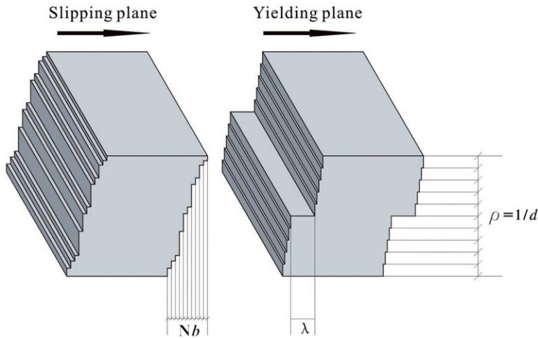
Figure 2. Schematic illustration of the contrasting patterns of plastic deformation for crystalline material (left,  $b$  stands for Burgers vector) and metallic glass (right).
