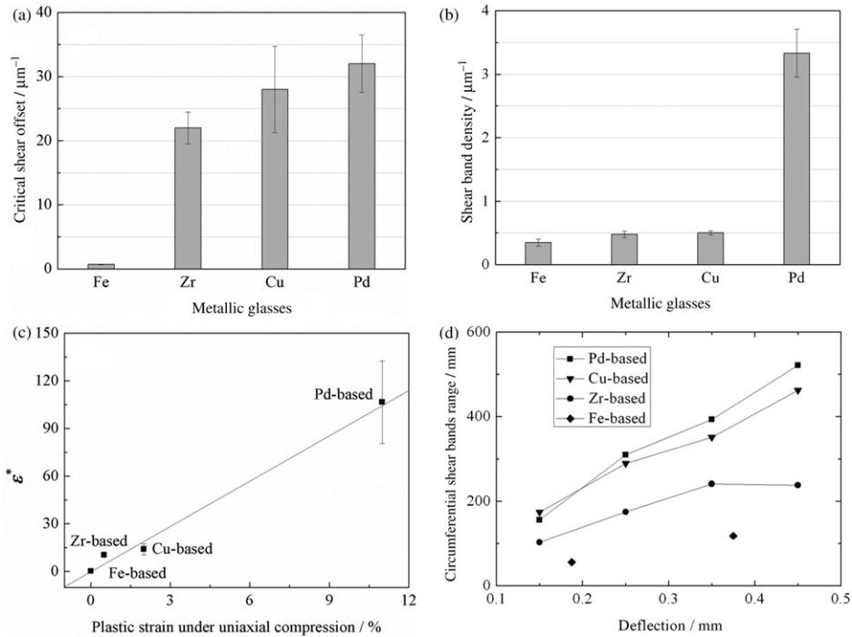
Figure 3. (a) Critical shear offset and (b) shear band density of metallic glasses with different plasticities; (c) correlations between macroscopic plastic strain (under uniaxial compression) and equivalent plastic strain  $\epsilon^*$ ; and (d) circumferential shear band range of the four metallic glasses at different deflection.
