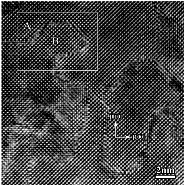
Figure 5. An HRTEM image showing the antiphase domain boundary structure. It can be seen that antiphase domain boundaries mainly lie on  $\{100\}$  and  $\{110\}$  planes. The white circuit is a rectangle, and the bottom left vertex of the rectangle does not lie on a bright image spot of domain B, whereas the other three vertices lie on bright image spots of domain A. Hence, it shows the relative shift between domain A and B.
