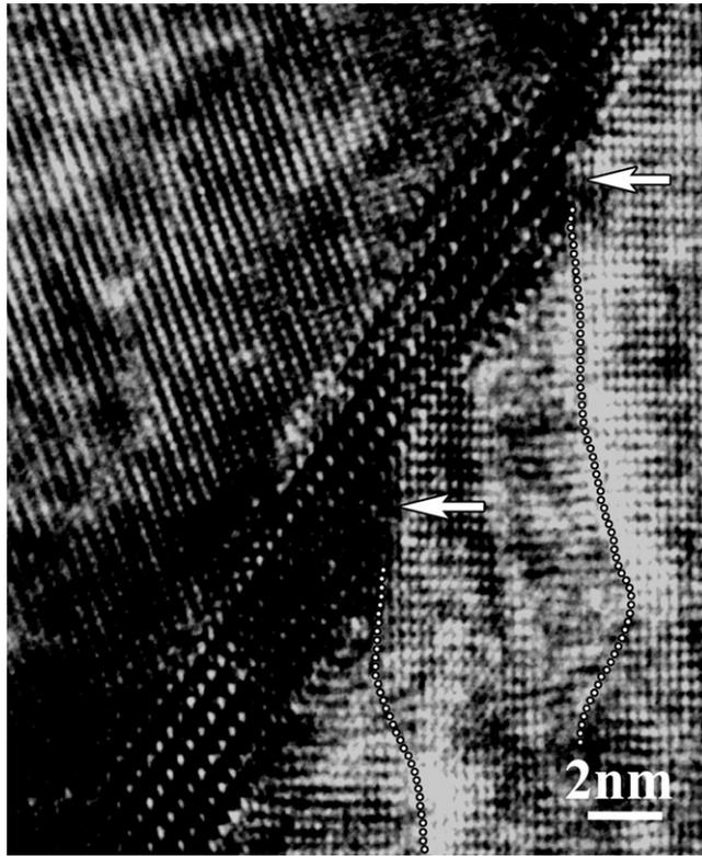
Figure 8. An enlargement of the region labelled by A in figure 7, which shows the details of the interaction of (111) twin and antiphase domains. Domain boundaries are indicated by dashed lines. Steps appear at the interaction areas pointed out by arrows.
