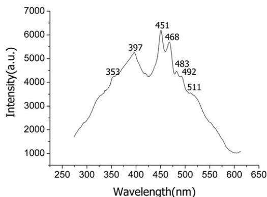
Fig. 4. Room temperature PL spectra of the SnO<sub>2</sub>/In<sub>2</sub>O<sub>3</sub> 1D nano-core-shell structures.
