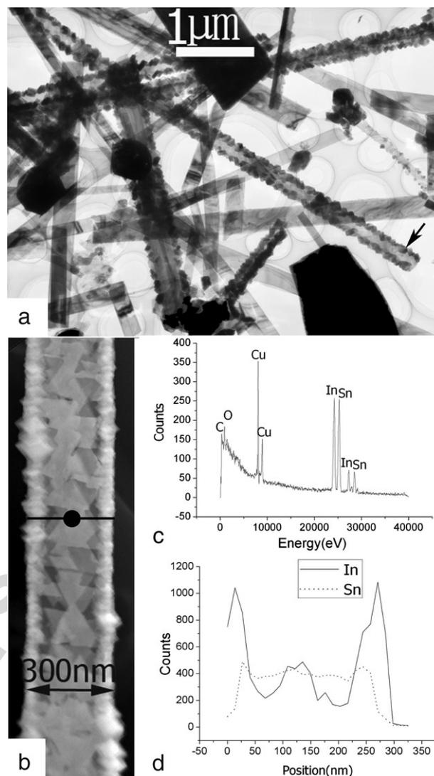
Fig. 1. (a) A TEM image shows the typical morphologies of the as-synthesized products, (b) A low magnification HAADF image of one of the  $\text{SnO}_2/\text{In}_2\text{O}_3$  1D nano-core-shell structures, (c) and (d) EDX analysis results corresponding to the point scanning and line scanning across the 1D nano-core-shell structure in (b).
