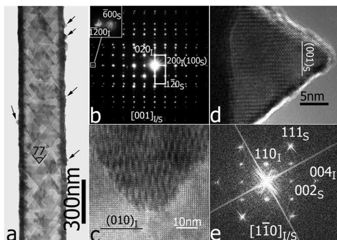
Fig. 2. (a) A low-magnification TEM image showing general characteristics of microstructures in the as-synthesized 1D nano-core-shell structures (b) the corresponding SAED pattern from the nano-core-shell structure in (a). (c) HREM image from the area marked in (a). (d) The HREM image corresponding to one of the ledges marked by arrows. (e) The FT pattern of the HREM image in (d).
