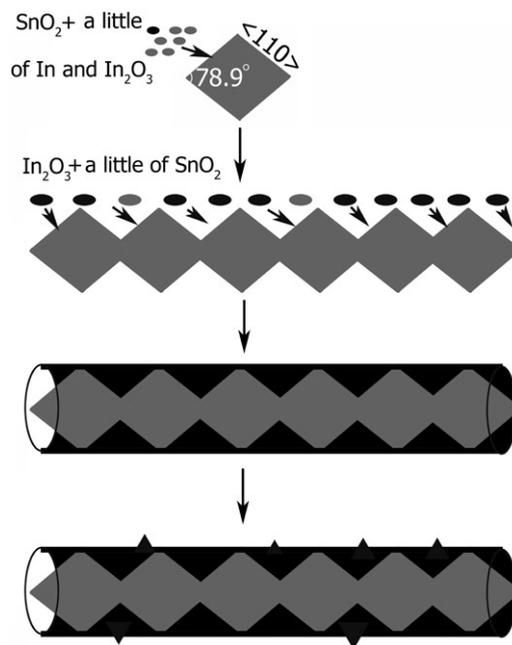
Fig. 3. Schematic illustration showing the possible growth process of  $\text{SnO}_2/\text{In}_2\text{O}_3$  1D nano-core-shell structures.
